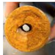
How iron contamination can affect a borehole if allowed to build up – a good reason to implement regular maintenance
